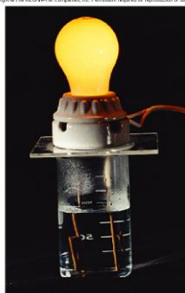
B Weak acid (or base) = weak electrolyte
