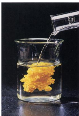
Figure 4.6 The precipitation of \text{PbI}_2 , a metathesis reaction.
