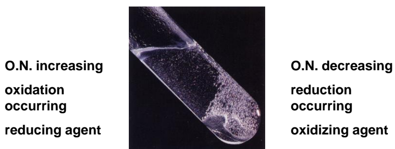
Figure 4.14 The displacement of H 2 from acid by nickel.
